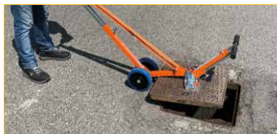
Use 1: opening with magnetic CL9 - CL10 - CL11.
