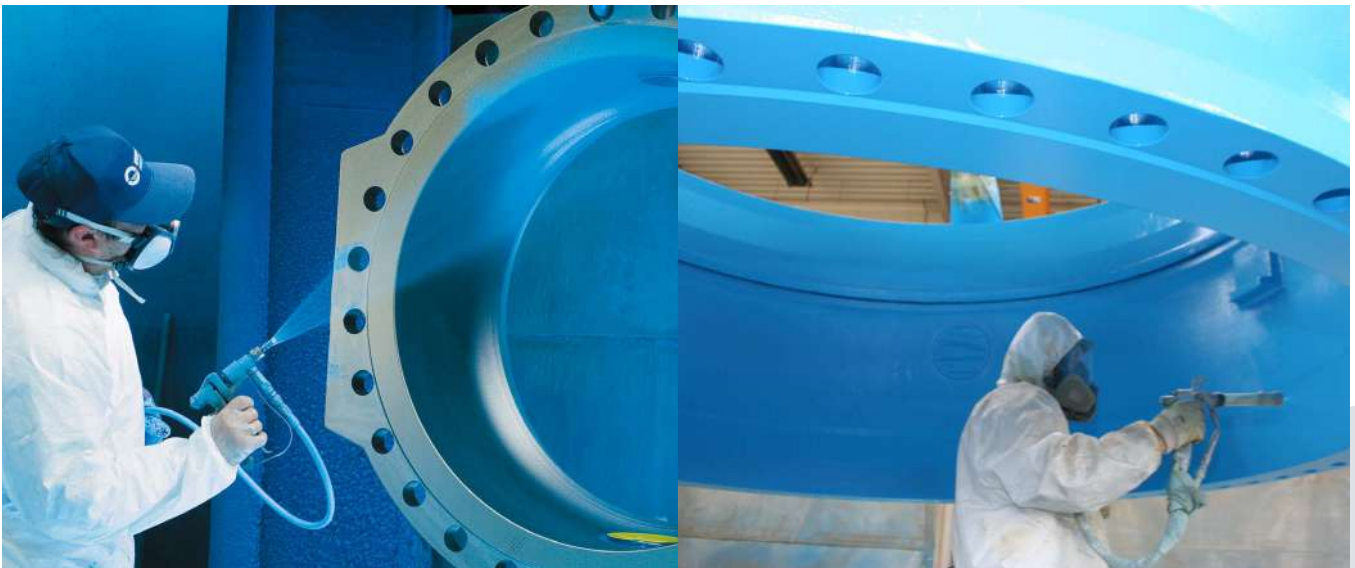
Epoxy coating at the ERHARD plant in Heidenheim / Germany
